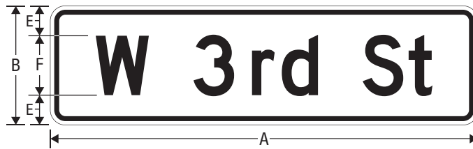
D3-1 STREET NAME (1 LINE, ALTERNATE COLOR ARRANGEMENT) OR
