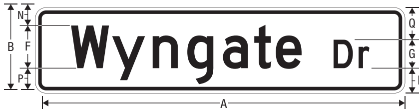
D3-1 STREET NAME (1 LINE, ALTERNATIVE COLOR ARRANGEMENT) PRINCIPAL LEGEND WITH DESCENDING STROKES
