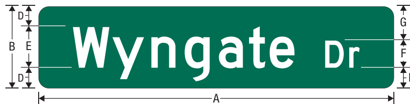
D3-1 STREET NAME (1 LINE) WITHOUT BORDER, PRINCIPAL LEGEND WITH OR WITHOUT DESCENDING STROKES
