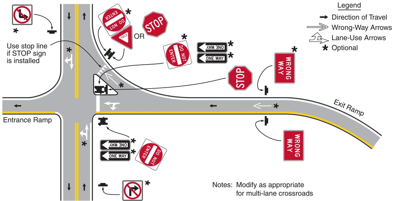
**Figure 2B-19. Example of Application of Regulatory Signing and Pavement Markings at an Entrance Ramp Terminal Where the Design Does Not Clearly Indicate the Direction of Flow**
