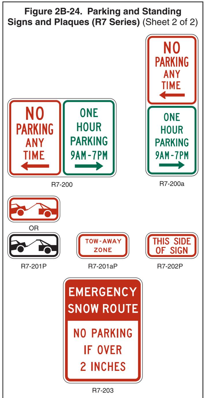
**Section 2B.47 Design of Parking, Standing, and Stopping Signs**
