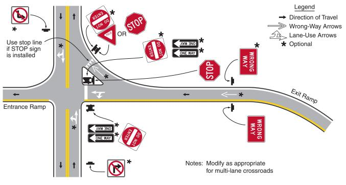
Figure 2B-19. Example of Application of Regulatory Signing and Pavement Markings at an Entrance Ramp Terminal Where the Design Does Not Clearly Indicate the Direction of Flow
