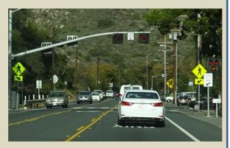
**Pedestrian-activated Warning Beacons** – Section 4L.03 describes the use of a flashing yellow warning beacon to supplement a pedestrian crossing warning sign. The warning beacon may be pedestrian activated to increase its effectiveness in making the crossing sign more conspicuous when a pedestrian desires to cross the roadway.
