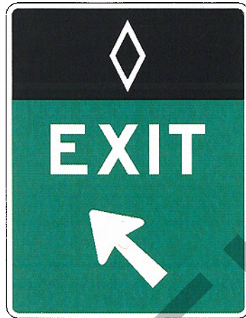
Fig. 3. Exit Gore sign at a direct exit from a preferential lane.
